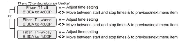
For one speed pumps, this is the first filter timeclock and will determine the normal hours of filtration for the pool. For pool/spa combination systems with spillover enabled, the valves will automatically switch to spillover mode at the start of the filtration period. For all other systems, the valves will switch to the pool-only position. Refer to the text above for general notes regarding timeclock programming.
