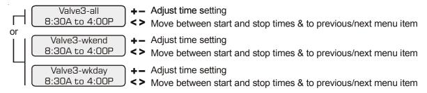
This menu will appear only if Valve3 is configured for timeclock. The valve will rotate on and off at the designated times. There is no manual override. If the Valve3 relay is on during the programmed off time, it may be because of freeze protection.
